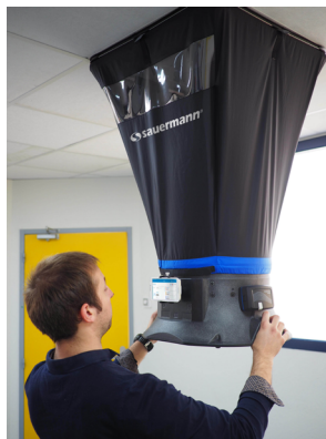
Air flow meter
