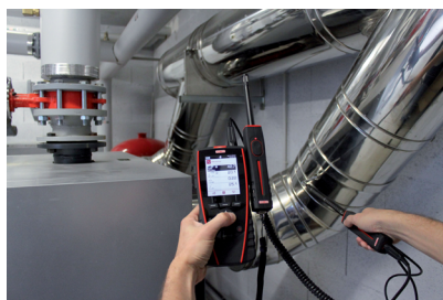
Hygrometry and air velocity measurement
